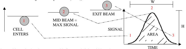
The resulting pulse has three measurable features: height, width, and area. Height = maximum fluorescence intensity. Width = transit time. Area = total fluorescence of particle.
