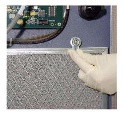
**4** Install a new filter and turn the pegs to hold the filter in place.
