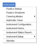
Fluidic control of the BD FACSCanto instrument is completely automated by BD FACSDiva software. The software contains pre-programmed fluidics protocols that are activated by choosing the corresponding command from the Instrument menu. In addition, fluid level indicators are available in the Instrument frame; see Fluid Level Indicators on page 48.
