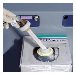
The cap, sensor and fluid lines, and the level sensor come attached in a single assembly piece.
