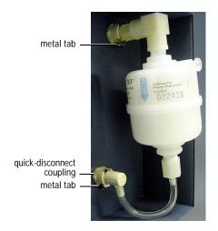
**3** Position the new filter and connect the couplings.
