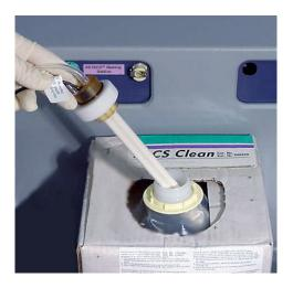
**5** Put a new level sensor assembly on the cubitainer or tank. Hand-tighten the cap until it is fully closed.
