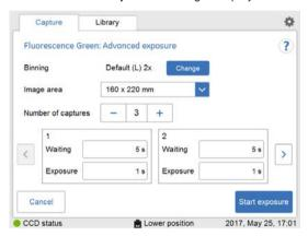
**Binning**, **Image area** and **Number of captures** can be specified depending on the conditions. The table below shows the available combinations.
