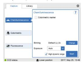
To change *Binning* from *Default*, click the *Change* button. The following pop-up screens will be displayed depending on if the sample tray is inserted in lower or upper position.
